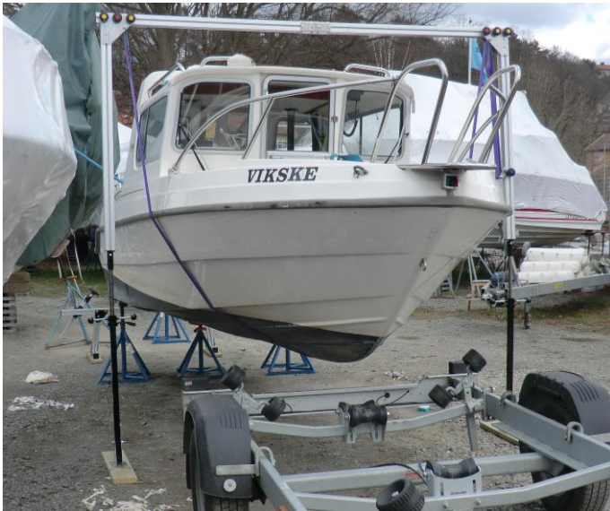
Picking up the boat after the trestle has been taking away.
